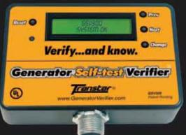
A 2x16 character LCD screen displays the status of over 15 functions and events and allows the user to enter all setup parameters.
